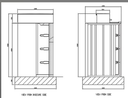
On receipt of a signal from a push-button, card reader etc., the turnstile will release the rotor, then closes and relocks. The park assembly has a positive action lock which prevents the arm rotating in reverse after 60°
